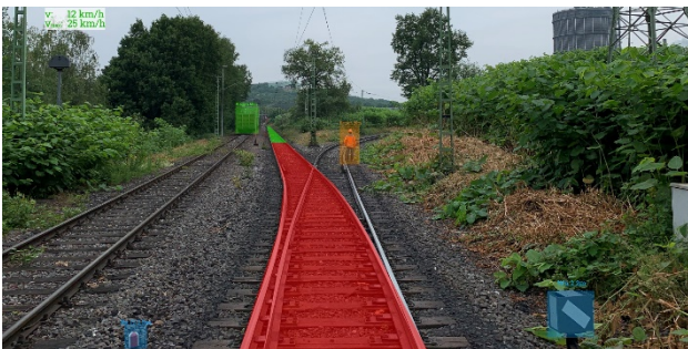
Figure 2. Augmented Reality in camera live stream highlighting persons, wagons, signals and the driveway including the braking distance.
