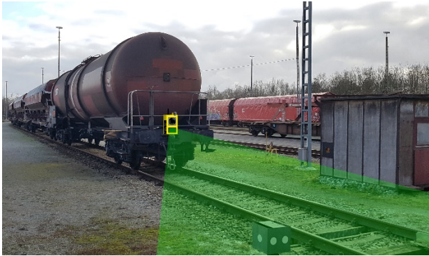
Figure 1. Sensor box attached to the train monitoring the track.
