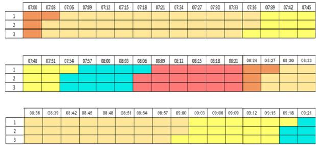
**Figure 4.** Section of heijunka of subassembly process of 5 different parts (represented with different colours, three work stations and process cycle time 3 minutes per part)
