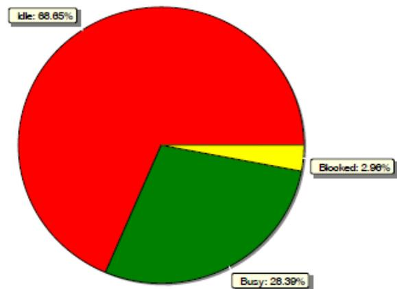
**Figure 2.** Utilization of the CNC lathe
