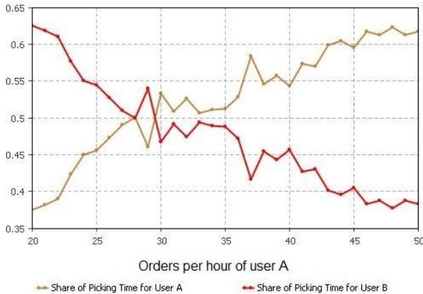
**Figure 2:** Picker time share for different numbers of orders per hour for user A with a fixed number of 30 orders per hour for user B.
