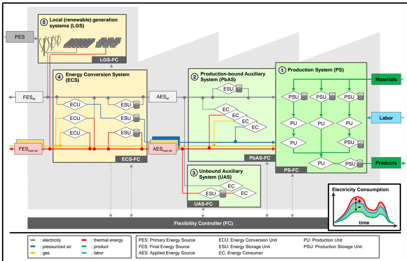
Figure 1: Flexibility controller in an energy-oriented PF
