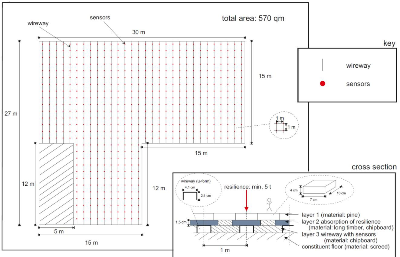
**Figure 2.** Layout of sensor floor
